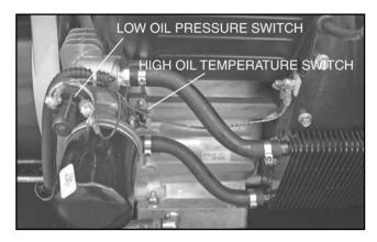
Figure 42. Oil Pressure Switch
